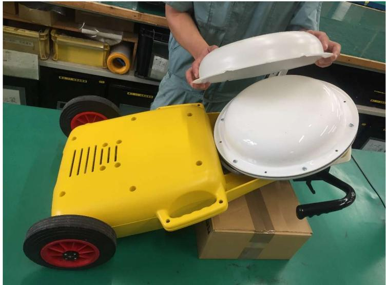
5) Return the 6 screws that were removed in step one and fasten the cover to the antenna
