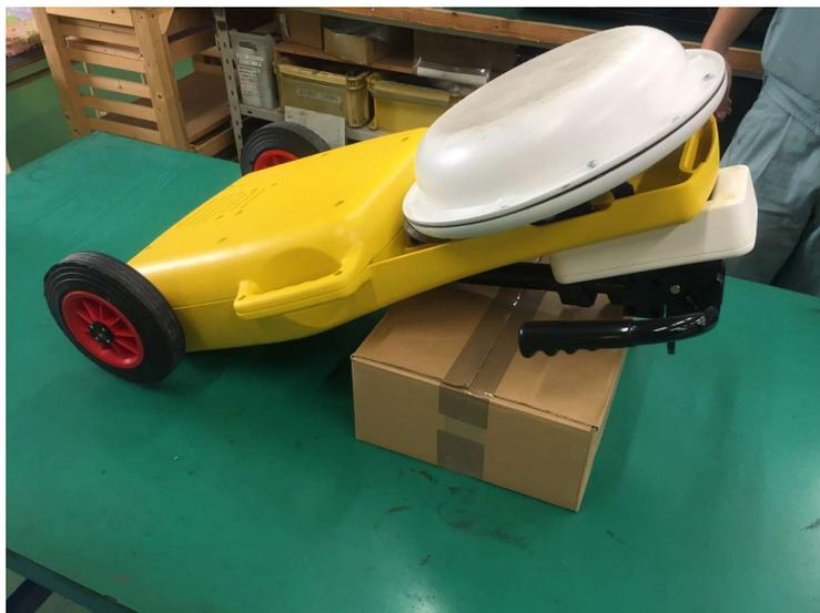
2) Using a Philips head (cross-head) screw driver, remove all 6 screws surrounding the antenna cover
