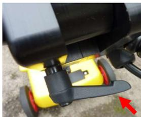
Please turn the coupling lever counterclockwise until the handlebar and the monitor move freely.
