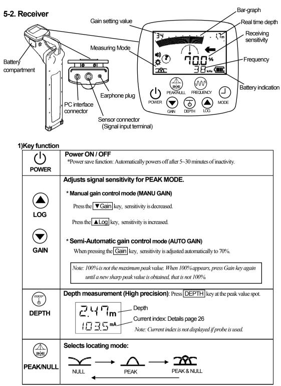
**PEAK & NULL MODE:** Maximum sensitivity is the point directly above the object line and the buried object line location is indicated with arrow.
