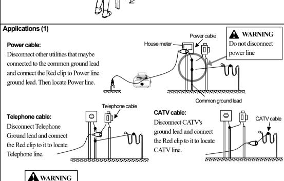
Remember to correctly reconnect common grounds for telephone & CATV. Check Local codes for proper grounding procedure. IMPROPER GROUNDING MAY CAUSE DAMAGE TO APPLIANCES, FIRE OR EXPLOSIONS.
