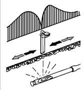
**Depth measurement**  $\Rightarrow$  Press | **DEPTH** | key
