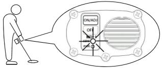
Detection of a metal cover is indicated by an audible pitch increase and SENS light brightness increase.
